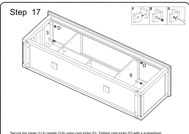
Secure top panel (1) to panels (3,6) using cam locks (D). Tighten cam locks (D) with a screwdriver.
